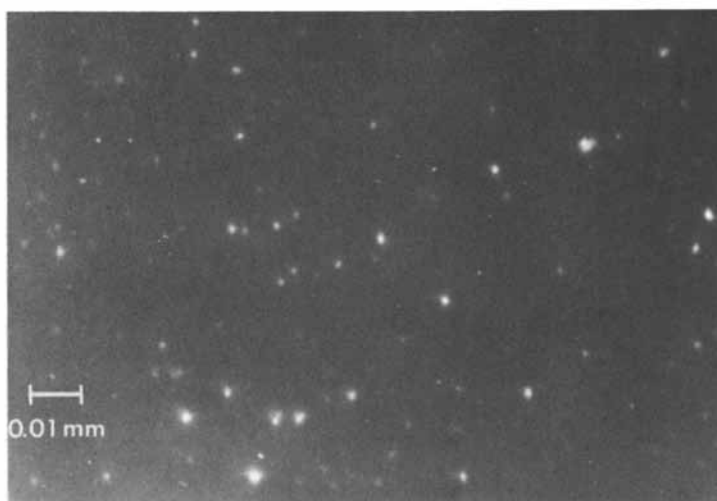
Figure 4. Polarizing optical micrograph of enamel made from 1c, 400 X magnification.
