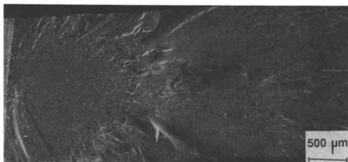
Figure 2b. Photon detector current as a function of time and corresponding fracture surface micrograph for rough fracture surfaces of TGDDM/DDS.
